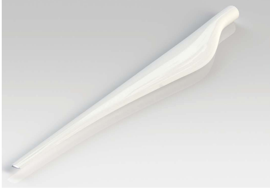
Figure 4.7- Completed blade formed from building lofted base from imported cross-sectional curves.
