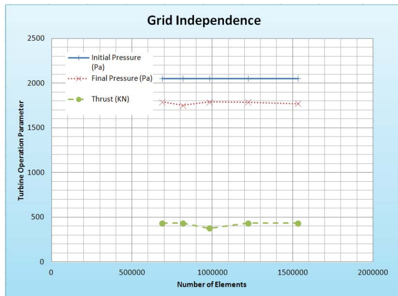
Figure 5.1- Grid Independence Study Performed so as to obtain convergence of Thrust and Pressure on the Turbine.
