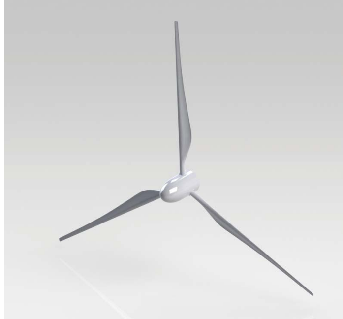
Figure 4.9- Completed rotor blade showing tri-blade setup connected to a center hub with face fillets.
