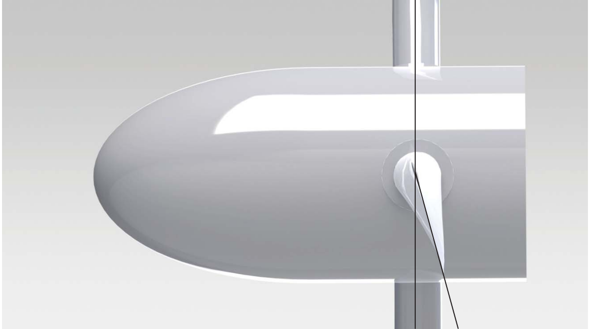
Figure 4.8 - Pitch angle of blade on model set at 15°.
