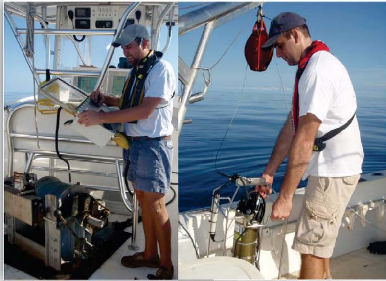
Figure 4.1- CTD Instrument setup onboard the Ocean Power preparing to collect data for temperature and salinity (Leland, 2009, p. 32).
